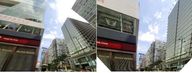
Fig. 4. Example of smartphone image captured with 45° pitch on the left, rectified image on the right.
